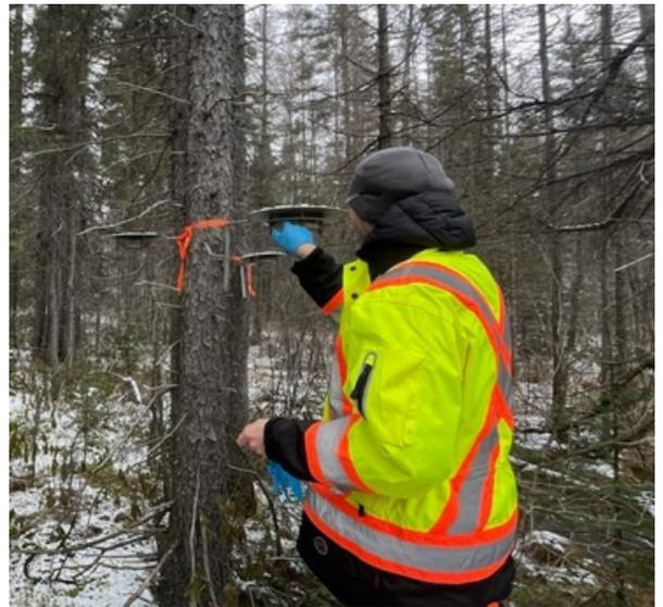
Opening of a dust sampler, Max Lakanen
